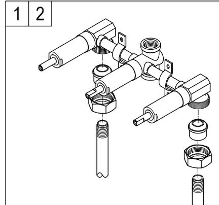
1. Properly secure valve body to wood bracing using copper straps. (not included)
