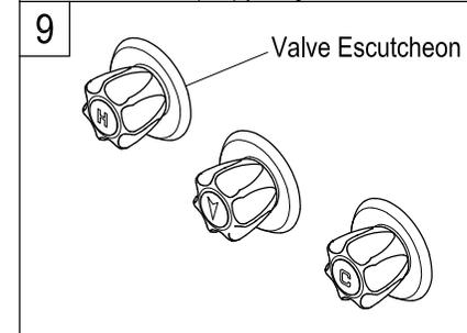
9. Remove handle. Push valve escutcheon over protruding valve assembly and secure with screws. Then replace handle.
