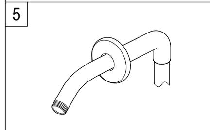
5. Place the shower flange over shower arm. Apply pipe compound to the threads on the long end of the shower arm. Screw that end into the shower riser elbow. Push flange against the wall.
