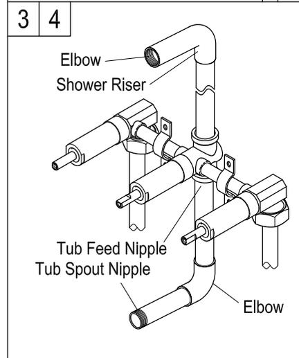
3. Assemble 1/2" elbow and 1/2" feed nipple. Screw into bottom of valve. Screw 1/2" tub spout nipple into elbow. Nipple should extend out from wall about 4-1/4." (If no shower is to be installed, use a 1/2" plug to close top opening of valve.)
