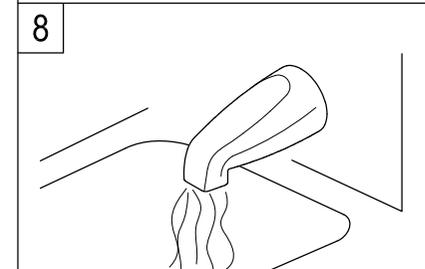
8. Turn on water supply and check connections for leaks. Place handle on valve stem and flush lines by running hot and cold water uninterrupted for one minute.
