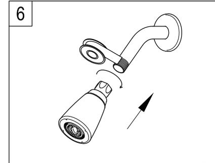
6. Wrap Teflon tape around all the threads on shower arm and hand tighten the shower head clockwise.
