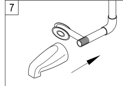
7. Apply pipe compound to tub spout nipple and attach spout to nipple. Hand tighten. Apply Teflon tape to inlet shanks and connect supply lines.
